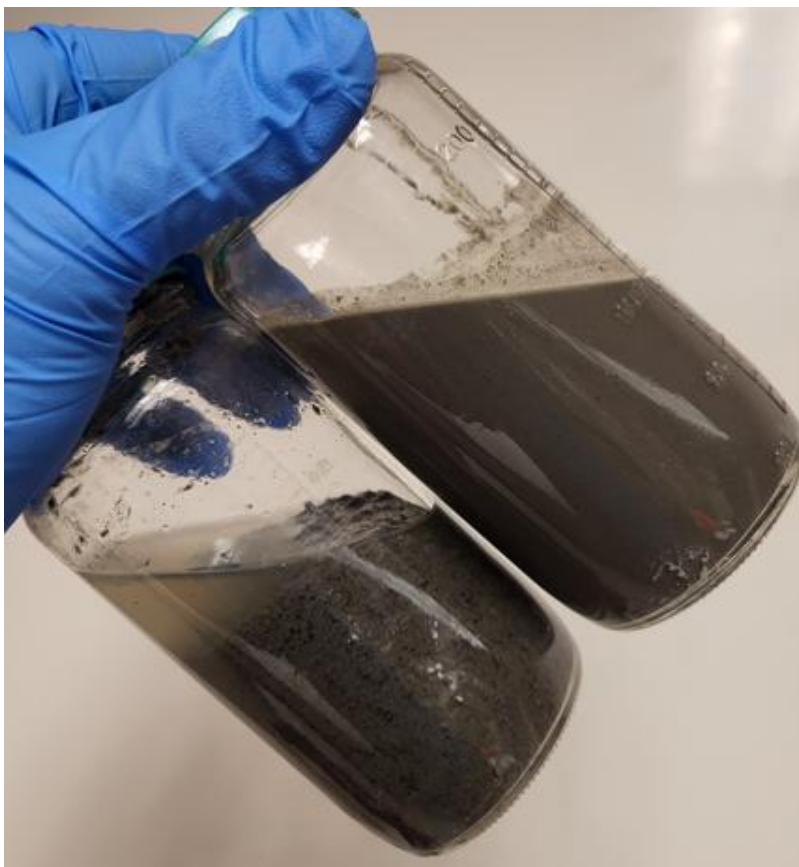
One hundred fifty milliliters of unconditioned sediment sample (top), One hundred fifty milliliters of sediment sample conditioned with Solve 164 (bottom).
